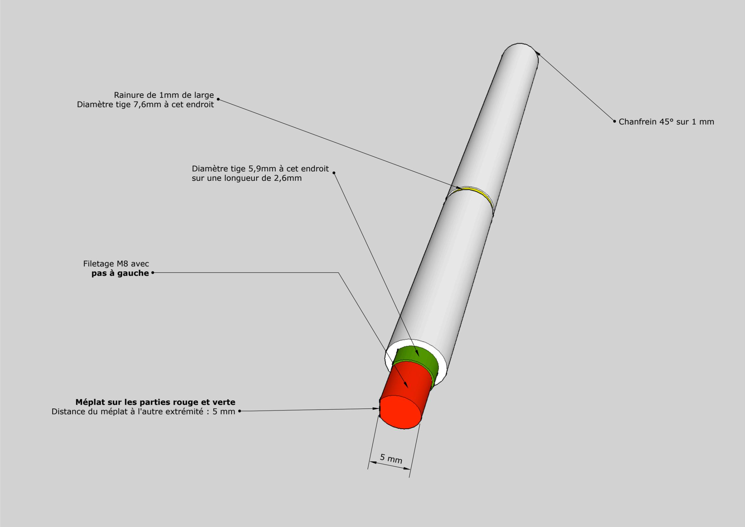
The diagram shows a shaft with several key features: a chamfered end (45° on 1 mm), a groove (1 mm wide, 7.6 mm diameter), a section of reduced diameter (5.9 mm diameter, 2.6 mm length), an M8 left-hand thread, and a chamfered end (45° on 1 mm). The shaft is shown in a perspective view, with a cross-section at the bottom showing a red and green section. A dimension line indicates a distance of 5 mm from the chamfered end to the other end of the shaft.
